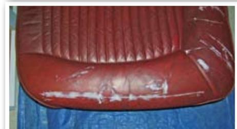
*Paste applied to help fill some of the cracks in the upholstery.*
