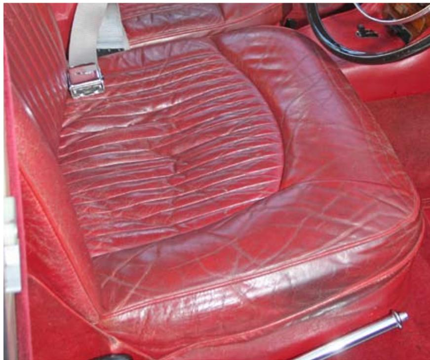
*The condition of the driver's seat when the car was purchased. No real damage but very dirty and the seat springing has obviously suffered over the years.*
