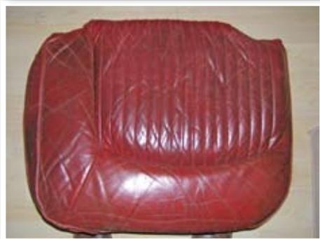
*The seat squab after adding the foam providing much better support and more of the original shaping.*
