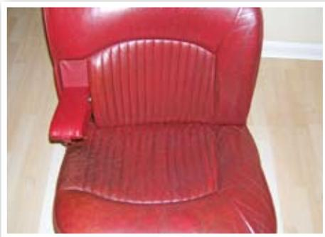
*The front passenger seat, prior to any refurbishment work. The very dark patches were the major areas of concern as the dirt and oils were heavily contaminating the leather.*
