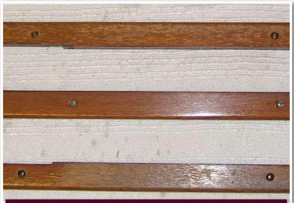
*The door cappings as removed from the car. Not in bad condition but the finish had deteriorated over the years with exposure to the light and heat.*
